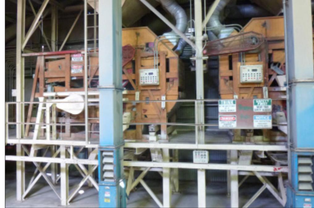
Existing equipment such as these Clipper airscreens are grandfathered into compliance with California's clean air standards. To replace the old machines would involve an extensive permitting process. Even if a permit would be granted, the associated fees would make it impractical to install new equipment.
