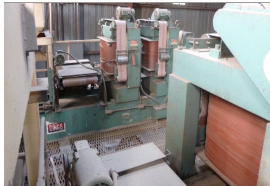
*Three two magnetic separators (mag mills) are useful for removing certain weed seeds. When fine iron powder is mixed with seeds, enough powder gets trapped in the weed seed's rough seed coat to enable the large magnet (red coils) to attract the powder and remove the weed seed. Similarly, the process also removes some alfalfa seed with cracked seed coat. (JWF photo)*
