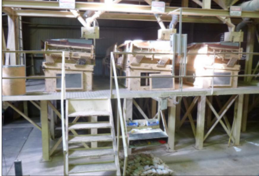
*Oliver gravity separators are components of S&W Seed Company's three processing lines for alfalfa, wheat, and small grains at its Five Points, CA facility. The facility is capable of processing 24 million pounds annually.*
